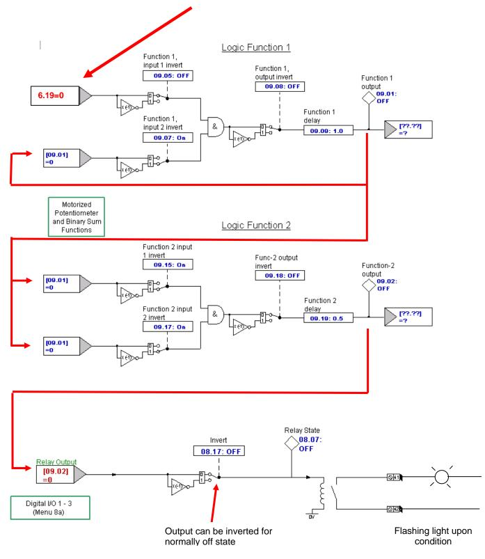
Obviously, if this relay is already in use, one could install an SM-IO Lite Module and perform a similar assignment. See page 3
