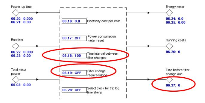
After maintenance is performed one could reset #6.19 back to Off which will reset the Hour meter and #6.27 will be at the number of Hours set in #6.18.
